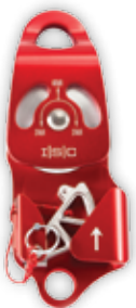
CE PCA-1271 Self-blocking pulley with aluminium side plates. 1 aluminium sheave 62 mm dia. For rope up to 13 mm dia. MBS: 40 kN
