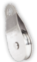
PCA-1275 Single swing side pulley with stainless steel plates. 1 aluminium sheave 76 mm dia. For 10 mm rope only. WLL: 16 kN
